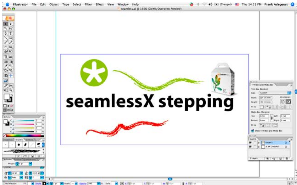
Design element that needs to be repeated on a seamless cylinder. The trim box, highlighted in blue, acts as the step and repeat reference cell.
