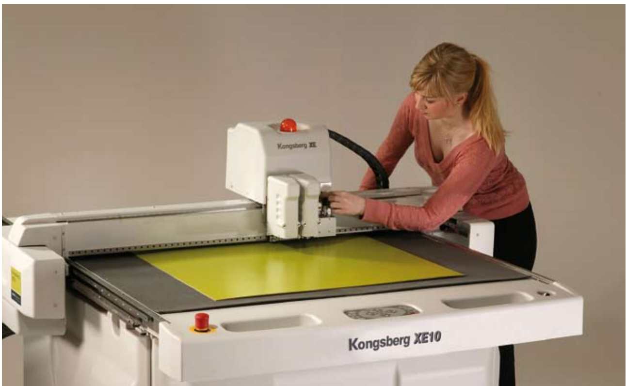
The Kongsberg XE10 is a small-format dieless digital table for cutting and creasing folding cartons. It is based on the technology and versatile architecture of the Esko Kongsberg XL tables, noted for their power and durability.
